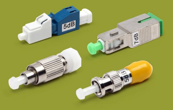
Fiber Optic Attenuators are used in the fiber optic communications to reduce the optical fiber power at a certain value, the most commonly used type is fixed male to female fiber optic attenuator, it has the fiber optic connector at one side and a female type fiber optic adapter at the other, inside, there is a piece of attenuation optical fiber, and the fiber optic attenuator name is based on the connector type and the attenuation value.
